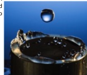
Chunlei Guo and Anatoliy Vorobyev developed a technique using lasers to render materials hydrophobic;. This photo by Adam Fenster was a top 10 finalist in the NSF Vizzies
